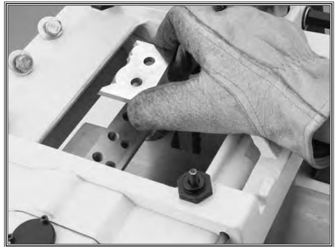
Figure 30. Moulder knife installation.
